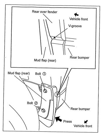
8. Press the mud flap (rear) in the direction of the arrow in the figure so that gap between the contacting surfaces at the upper/lower area of the V-groove are uniform. Securely tighten bolt ① so that there is no gap in the contacting surfaces with the rear over fender.
