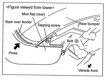
9. While pressing the mud flap (rear) in the direction of the arrow in the figure, securely tighten the tapping screw so that there is no gap between the contacting surface of the rear over fender.
