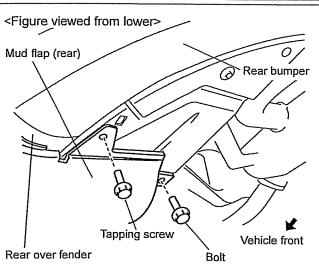
7. Set the mud flap (rear) to the rear over fender and temporarily tighten the bolts and tapping screw.
