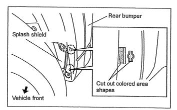
4. Cut out the colored area shapes in the two locations shown in the figure using nippers.
