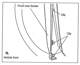
5. Remove the front over fender clips in the three locations from the bottom.
