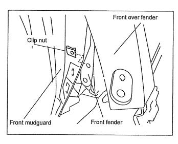
Peel back the front mudguard and front over fender, and install the clip nut to the position shown in the figure of the front fender.
