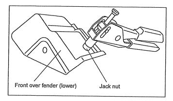
Install the jack nut to the hole on the underside of the removed front over fender (lower).
