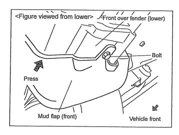
12. While pressing the mud flap (front) in the direction of the arrow in the figure, securely tighten the bolt so that there is no gap between the contacting surface of the front over fender (lower).
