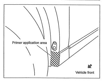
After removing the oil from the area of the front over fender (lower) shown in the figure using IPA or white gasoline, let it dry sufficiently, and then apply primer.
