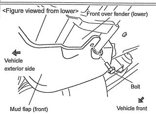
Remove the paper backing from the double-sided adhesive tape on the mud flap (front), and temporarily tighten the tapping screw and bolt.
