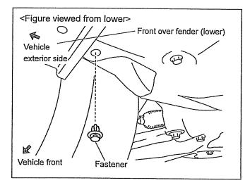
2. Remove the fastener on the underside of the vehicle body shown in the figure.
