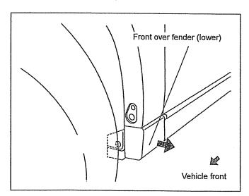
Grasp the flange on the vehicle interior side of the front over fender (lower) with your hand, pull it in the direction of the arrow and remove it. (Front over fender (lower) is secured by tabs in three locations.)
