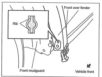
6. Cut out the rib of the front over fender shown in the figure using a nipper.
