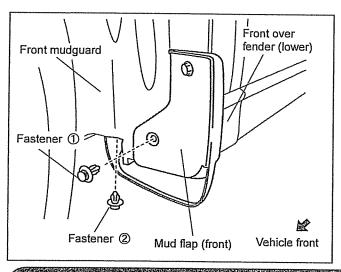
13. Install the mud flap (front) using the fasteners in the order of fastener ① and fastener ② shown in the figure.
