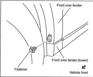
Re-install the front over fender and front over fender (lower) to their original positions and only install the one reusable fastener removed in Step 1.
