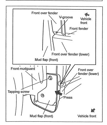
11. Press the mud flap (front) in the direction of the arrow in the figure so that the gap between the contacting surfaces at the upper/lower area of the V-groove are uniform. Securely tighten the tapping screw so that there is no gap in the contacting surfaces with the front over fender and front over fender (lower).
