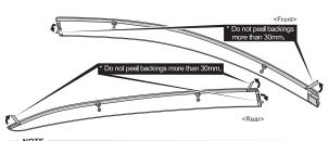
Do not peel the adhesive tape backings more than 30mm, as this will make it impossible to move the acrylic visors when positioning them correctly.
