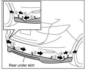
11.Peel off the paper backings of the double-sided adhesive tape in the direction of the arrows and press the tape against the body with sufficient force.
