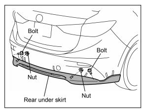
10.Attach the rear under skirt to the vehicle and temporarily install it using the nuts (2) and bolts (2).
