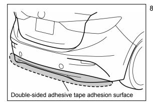
8. Apply pack primer to the unpainted bumper surface area where the double-adhesive tape is to be adhered.
