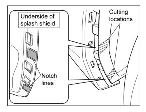
Use a nipper or utility knife or similar to cut the splash shield along the notch lines on the underside of the splash shield.
