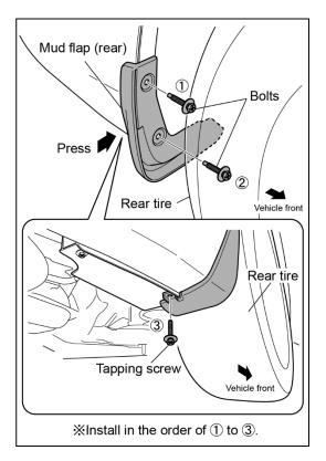
9. While pressing the mud flap (rear) against the rear bumper as shown in the illustration so that there are no gaps, install it by using the bolts (2 places) and the tapping screw (1 place).
