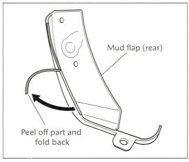
12. Peel off part of the backing paper from each piece of double-sided adhesive tape on the mud flap (rear) and fold them back.
