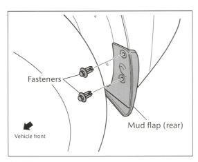
5. Set the mud flap (rear) against the vehicle, and then install the fasteners (2 places).
