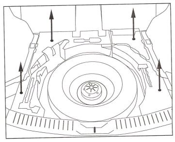
3. Remove 2 trim pannel fasteners and pull directly up to remove threshold and set aside.
