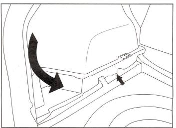
5. Being careful not to damage clips, partially remove the lower interior trim panels on each side of the vehicle. Locate the vehicle's taillight wiring harness.
