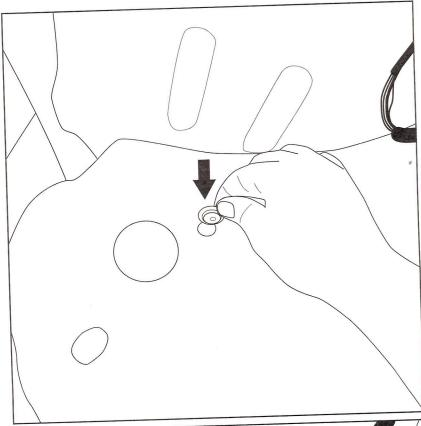
17. From underneath the vehicle feed exposed terminal end of the 4-flat harness through the grommet and seet grommet.
