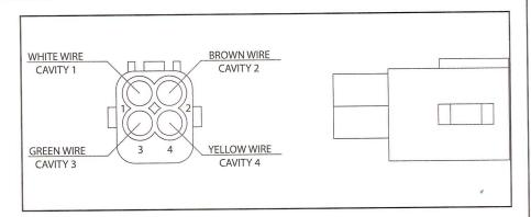
19. Connect the 4-Flat Harness to the mating end of the trailer tow harness. All connector surfaces should be clean and free of dirt.
