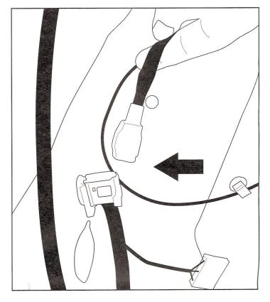
7. Insert the short T-Connector end between the vehicle connectors. Be sure that connectors are fully inserted with locking tabs in place. All connector surfaces should be clean and free of dirt.
