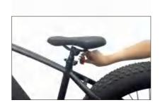
Insert rear light into the retaining clip
