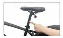
**02**Adjust the height to be suitable, and pay attention that the seat pipe does not exceed the minimum safety line
