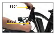
$02\,$  Fix the front shock absorber and rotate the riser 180  $^{\circ}$
