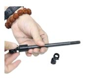
Insert the bearing screws into the corresponding holes in the front tire
