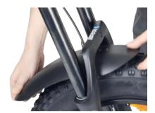
Use a tool to tighten the screws to secure the front fender into the middle of the front fork
