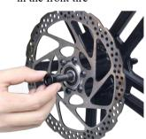
Lift the body and align the front fork with the bearing screws on the front wheels
