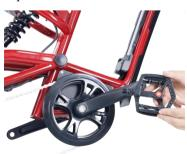
By turning the right pedal clockwise and the left pedal counterclockwise with your hand,Use tools to tighten pedal
