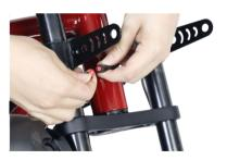
Place the screw in the side hole of the headlight
