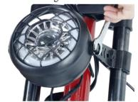
Remove the screws in the center of the front fork
