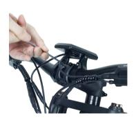
Tighten the two screws on the riser to secure the head pipe
