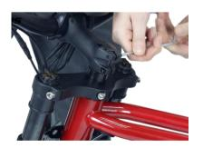
Remove the screws under the rear shock absorber
