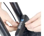
Align the front fender with the hole on the front fork
