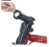
Place the handlebars into the corresponding lock mouth
