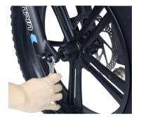
Install the nut on the other side to the bearing and tighten the nut
