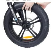
Put the front fork on the bearing screw and find the matching nut
