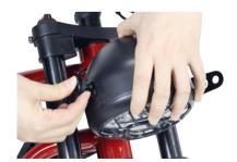
Tighten the screws on the left and right sides of the headlights
