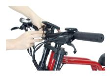
Use a tool to tighten the four screws at the lock opening to secure the handlebars
