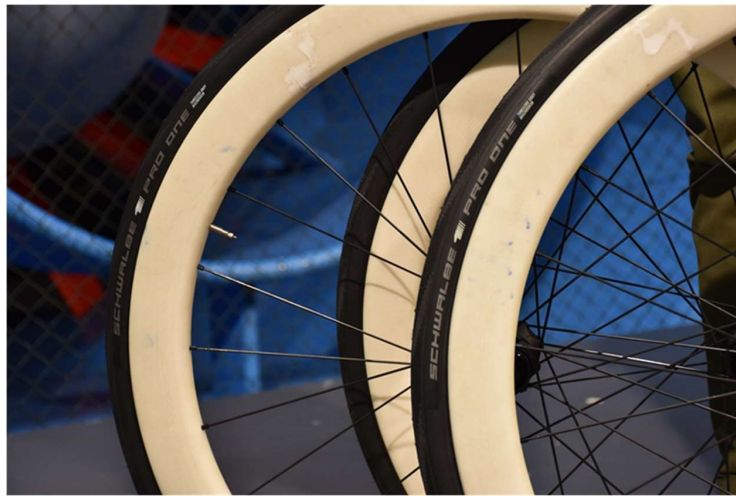
Figure 5 Photograph of the 3D printed ABS prototypes
