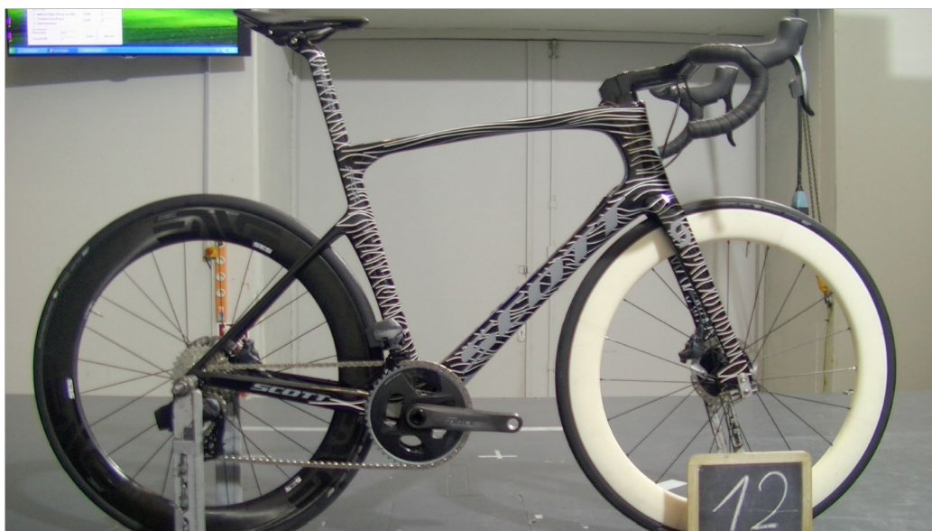
Figure 5 Photograph of the 3D printed ABS prototypes during the prototype Wind Tunnel Test
