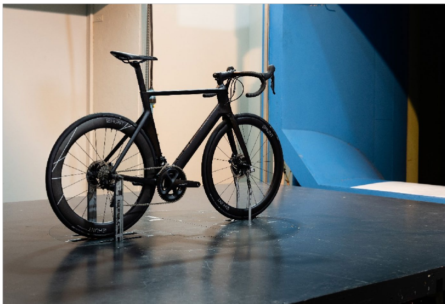
Figure 3 Wind Tunnel Setup (60 Limitless Rear / 48 Limitless Front)
