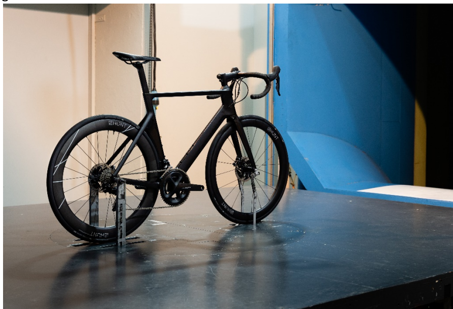
Figure 3 Wind Tunnel Setup (60 Limitless Rear / 48 Limitless Front)
