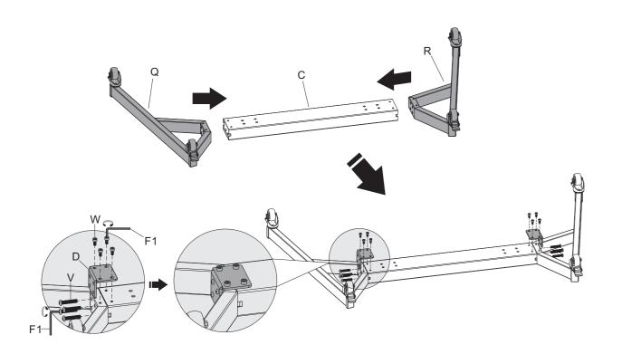
Insert the right leg into the base. Align the holes in the right leg to the holes in the base. Secure with the connecting pieces and the screws. Repeat this step for the left leg.
