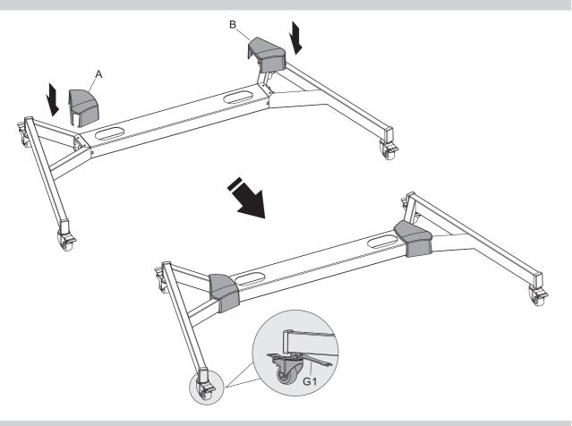
**NOTE:** Lock the brakes on the casters to avoid any sudden movements during installation. Each caster can be adjusted independently for fine tuning. Slightly turn the nut to lower or raise the base.
