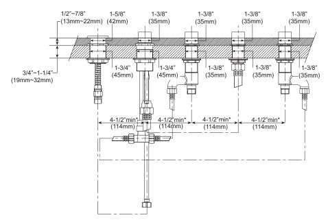
IMPORTANT NOTE: This valve/trim can only be installed in a built-up deck. It cannot be installed on pre-finished deck or on tub rim.
