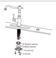
2. Adjust the position of the faucet and secure it with the fixing kit as photo.
