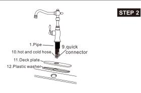
Position the faucet, deck plate and o-ring on the installation surface.
