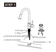
1.Position the faucet,o-ring on the installation surface.And then put the faucet into center hole.
