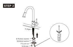
2.Adjust the position of the faucet and secure it with the fixing kit as photo.
