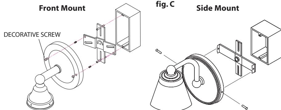
**\*Note:** If your fixture has a sliding backplate loosen the set-screw and slide the backplate toward the socket (be careful not to scratch the finish). Mount the fixture to the box and wire the fixture as described in section B. When finished, slide the backplate against the wall and tighten the set-screw.
