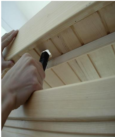
FIG-13 Slip cords/wires through corresponding holes
