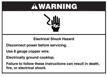
This cooktop is manufactured with a frame connected, green or bare ground wire. Connect the cooktop cable to the junction box through the UL listed or CSA approved conduit connector.
