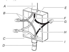
A. 3-wire cable from power supply B. Red wires
