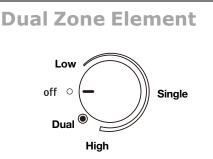
The dual zone elements offer flexibility depending on the size of the cookware. Single size can be used in the same way as a regular element. The dual sizes combine single and dual elements and are recommended for larger cookware, large quantities of food, and home canning.
