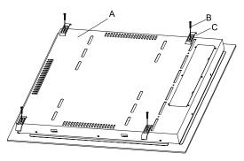
A. Cooktop base bottom B. Clamping screw C. Clamping bracket
