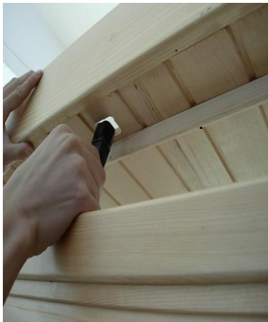
FIG-12 Slip cords/wires through corresponding holes
