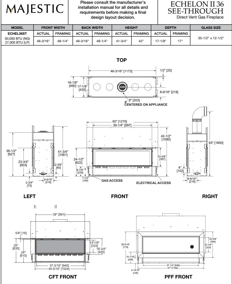
The PFF decorative front has an installed depth of 3/4" [19mm], measured from the front of the non-combustible finishing material to the front of the decorative front.
