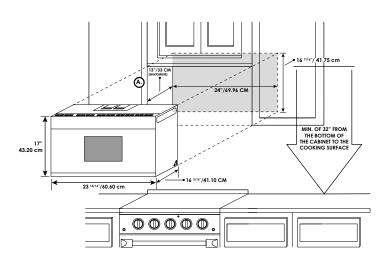
**A.** If the cabinet depth including the cabinet doors is more than 13"/33 cm then the unit must be spaced out from the wall using adequate materials supporting 150 lbs to allow proper top vent air exhaust/intake.
