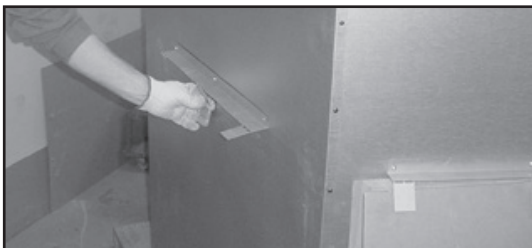
Figure 3.7 Bending Refractory Shipping Tabs Back Down
