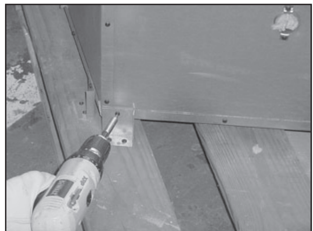
Figure 3.12 Removing Shipping Brackets
