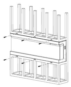
8. Cover the glass panel with protective plastic bag and install plywood or drywall.
