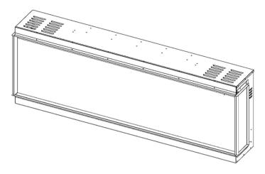
2. Remove the 7 screws on the left side. Take off the fending bar and panel.
