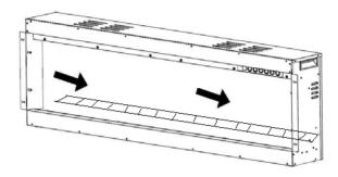
**8.** After placing the Decorative Crystals or Pebbles on the designed slot, fasten screws back on the glass panel and the metal trim.
