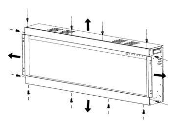
7. Place the top and bottom trims on the appliance and fix them using the screws removed in the previous step.
