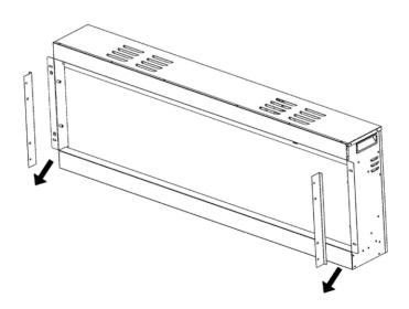
**5.** Place the left and right trims on the appliance and fix the part using the screws provided in the kit.
