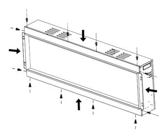
8. Put the appliance into the wall opening and fix it with the screws provided.
