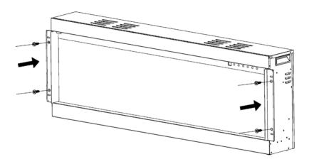
**6.** Remove the relevant screws at the top and bottom of the appliance.
