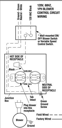
\*An ON/OFF Wall Switch is used with the FBK-100 kit (field provided or sold separately - order P/N 85L87); A Variable Speed Control (provided) is used with the FBK-200 kit. The installation of these kits also require a Junction Box / Electrical Kit (provided).
