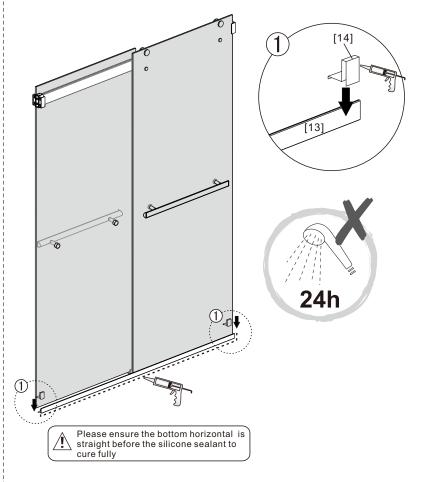
Do not use the shower enclosure for at least 24 hour in order to allow the silicone sealant to cure fully.
