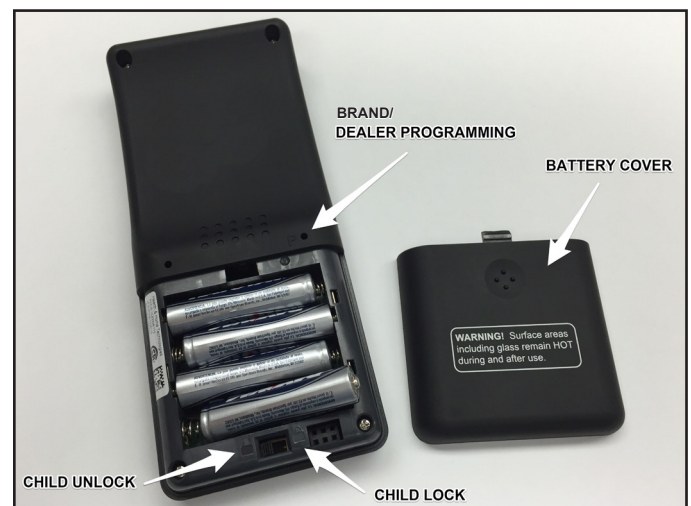
Figure 1. Install Batteries & Child Safety
