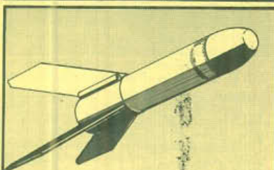
1. Featherweight Recovery (i.e. Astron Streak): The model is designed for extra light weight (under 1/4 ounce without engine) and has a blunt nose. When the engine is ejected from the rocket, the model is so light compared to its size that it lands safely. The lightweight, aerodynamically unstable, spent engine casing tumbles back separately.
