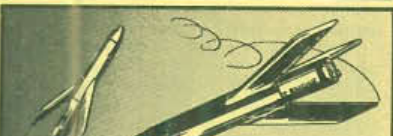
2. Tumble Recovery (i.e. Astron Scout, Sprite): The ejection charge shifts the weight of the engine in the rocket rearward. This makes the rocket unstable. With the balance point of the rocket further toward the rear, air pressures ahead of the balance point are greater than behind, forcing the rocket to start turning. When the rocket is tumbling, air drag on it is much higher and it falls slowly. Estes Pat. No. 3,114,317
