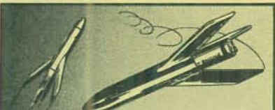
2. Tumble Recovery (i.e. Astron Scout, Sprite): The ejection charge shifts the weight of the engine in the rocket rearward. This makes the rocket unstable. With the balance point of the rocket further toward the rear, air pressures ahead of the balance point are greater than behind, forcing the rocket to start turning. When the rocket is tumbling, air drag on it is much higher and it falls slowly. Estes Pat. No. 3,114,317
