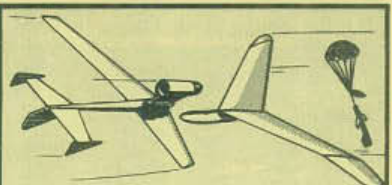
6. Glide Recovery (i.e. Astron Falcon, Nighthawk): The model ascends vertically like a conventional rocket. At ejection either the balance of the model or the position of its aerodynamic surfaces is changed. Instead of streamlining straight down, the wings generate lift, pulling the nose up, and the model goes into a glide. Models of this type are called "Boost-gliders". Estes Pat. No. 3,157,960. Other pat. pending.
