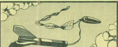
3. Streamer Recovery (i.e. Astron Mark): A model with a small streamer will act like a tumble model. If the streamer is large enough, it develops enough drag by fluttering to actually hold the rocket back in its descent and it lands gently.
