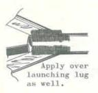
GAUZE REINFORCING: For super strong fin joints, reinforce with this unmarked gauze. Comes in 3" x 12" sheets. Apply by spreading a thin layer of glue over the area to be reinforced, smooth gauze down over the glue, and spread one or more layers of glue over the gauze. Shipping weight 1 oz.
