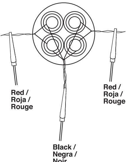
**Caution:** Examine all connections carefully. Be certain that the clips do not touch one another or the metal blast deflector. Be certain that none of the twisted starter lead bundles have loosened. If so, disconnect the clips, remove the rocket from the launch pad and re-twist the starter leads. /
