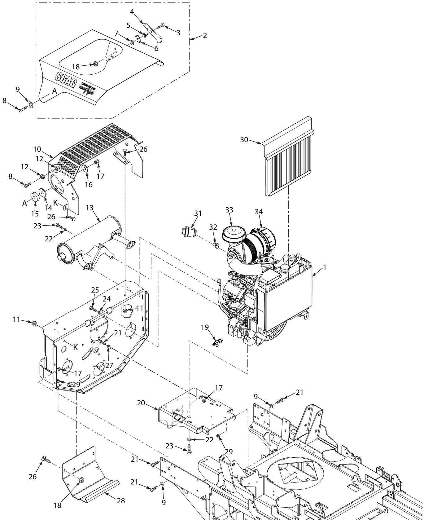
**STTII ENGINE & ATTACHING PARTS - LIQUID COOLED (GASOLINE)**
