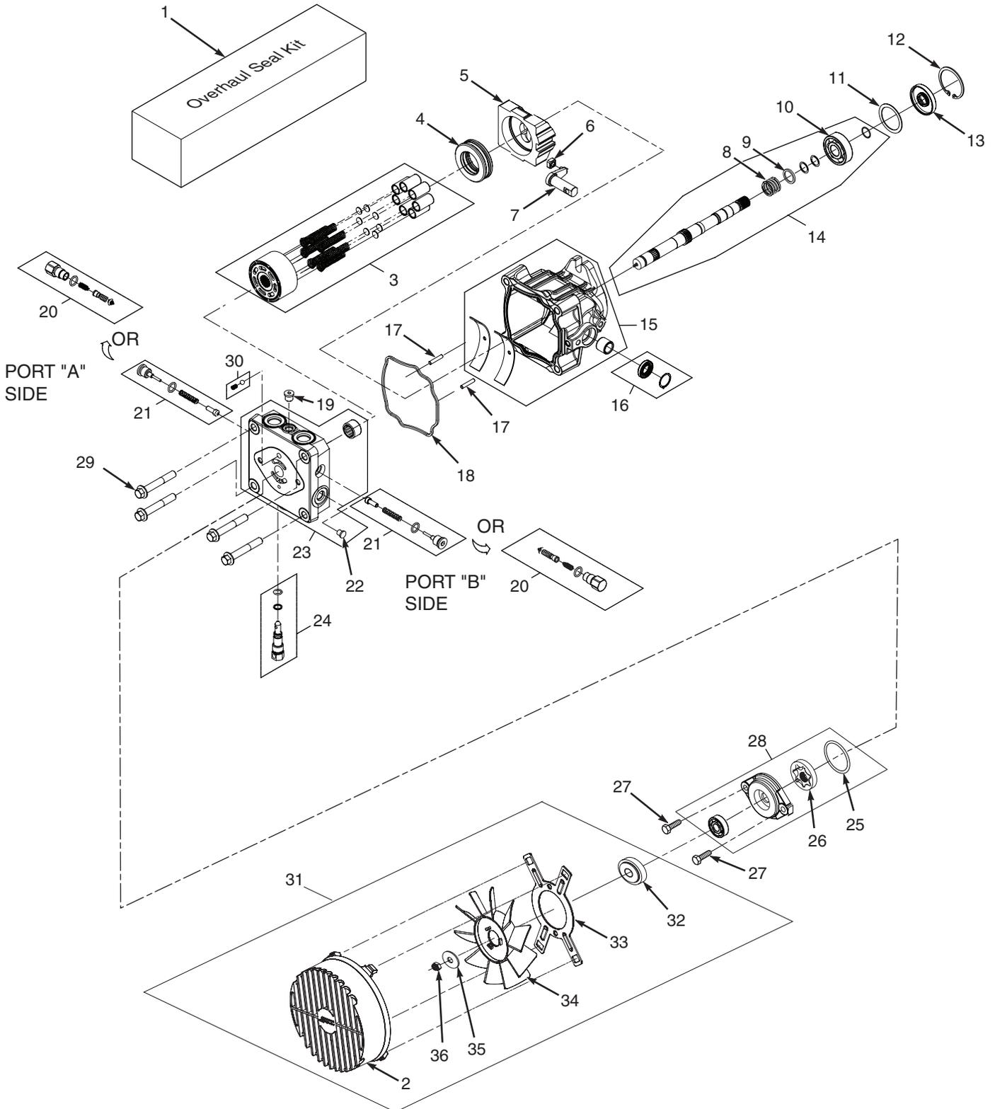
**BDP-16A HYDRAULIC PUMP ASSEMBLY with COOLING FAN**
