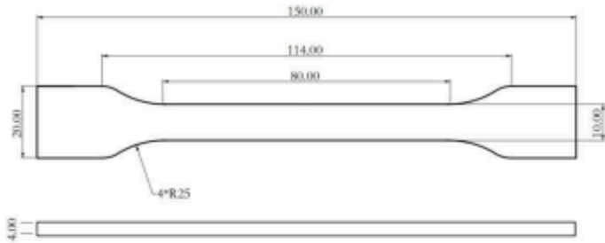
Tensile testing specimen; ASTM D638 (ISO 527, GB/T 1040)
