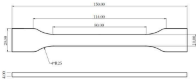
Tensile testing specimen; ASTM D638 (ISO 527, GB/T 1040)
