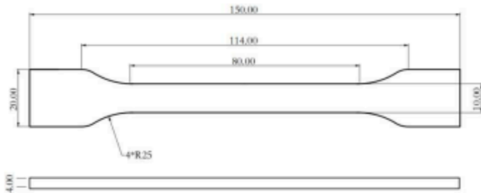
Tensile testing specimen; ASTM D638 (ISO 527, GB/T 1040)
