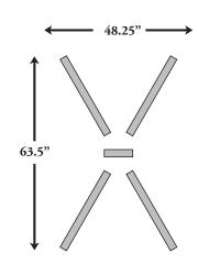
**For maximum wind resistance:** All four (4) legs must be in the down and locked position when using either 36"x36" or 48"x48" roll-up signs
