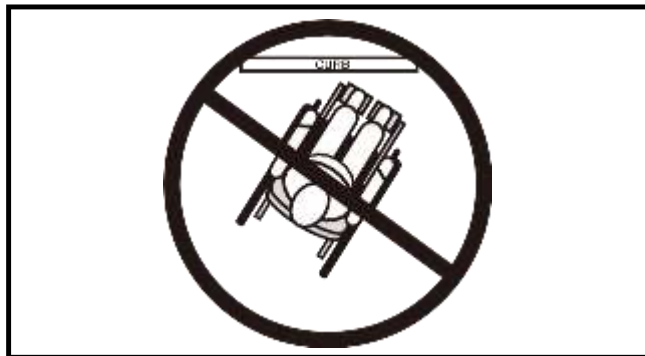
Figure 3. Incorrect Curb Approach
