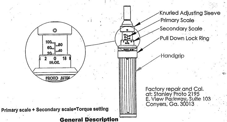
Your torque screwdriver complies to ANSI standard B107.14M, Type 3, Class A, Style 1.
