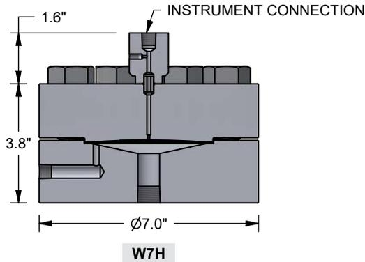
**Note:** All drawings depict a single 1/4" NPT Flush Port (optional). Drawing are not to scale. Contact Reotemp customer service for more detailed drawings. All dimensions are nominal
