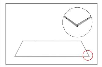
**Step 4:** Unzip print and lay image face up. Slide print onto frame like a pillow case. Grip the fabric tightly and stretch around bottom pole to pinch zipper into place. Zip the graphic together for taut finish.
