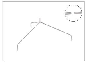
**Step 3:** Install bottom feet by joining two panels together and inserting dual posts into bottom of frame corners. Install connector clips between panels for stability. (x3)
