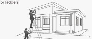
Determine the position of the first string of lights. Make sure that the adapter and control box are long enough to connect to the power supply. Fix the adapter to the wall to reduce the burden on the string lights.
