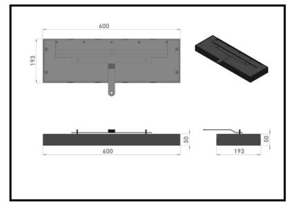
Above : The overall sizes of the burner tray. Below : The Single and Double Sided Enclosure (sizes below)
