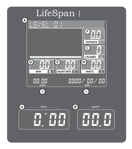
A. Alpha Numeric Window - The C7000i comes with a 16 character alpha window that is used to show the program name and set user functions like date and time.
