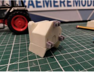
**3** Assemble the body. Glue the chassis to the leg frame with the legs slanting away from the linkage. If you want the chute to be fixed also glue that in place. If you want it to rotate leave it unglued and paint
