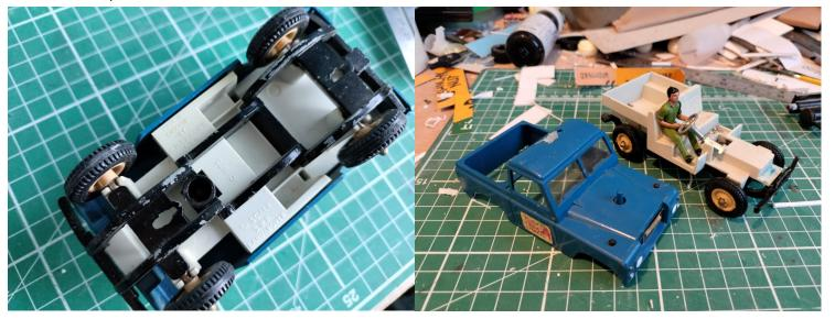
**2 Remove glazing.** If still present slide the glazing out. Push the plastic sheet back into the cab and then pull from one end through the side window as illustrated.
