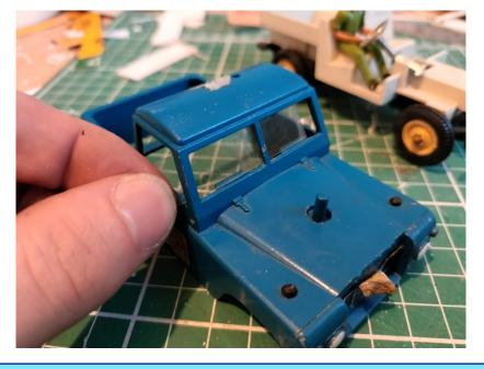
**3 Cut the cab off.** Remove the existing cab structure. **TAKE EXTRA CARE**, these are 50 year old diecast models, the material is weak and brittle. I use a combination of Dremel and handsaw to cut the roof away. Cut just above the windscreen and door line as illustrated.
