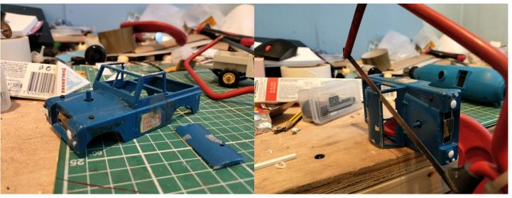
**4 Prep for new parts.** Although not necessary we stripped the old paint for a better final finish. Wilkos paint stripper scrubbed with a wire brush and left overnight wrapped in tinfoil. Also file the cut lines on the cab so they are flat and square ready to receive the new roof.
