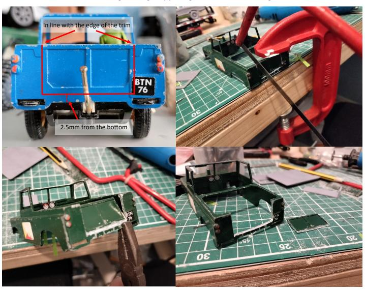
**6 Door and sides on.** Sand any lips left over from printing away. Glue the door inplace, ensure the back is flush with the metal as the plastic interior has to fit back in. The glue the two sides in place. Sand the flat faces of the side smooth to remove the print layer marking which will show up through paint.
