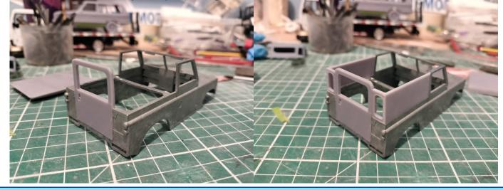
**7 Add the roof.** There is a slight lip left over from printing on the inside of the door cut out in the cab. This needs sanding or cutting away so the door fits correctly. Simply glue the door ontop ensuring the door cut out lines up and everything is neat and square.
