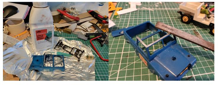
**5 Cut the door cavity.** Using the door as a template draw out the cut lines for the door. See the illustration for where to cut. To actually cut the space we used a hacksaw to cut down the sides of the tailgate, then slit the bottom with a Dremel and snapped the tailgate out. Finally we filed the cut out square checking all the time until the door was well received checking the height by placing the roof on and making sure it sits flat.
