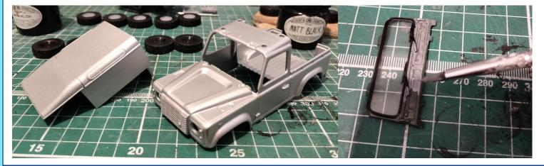
**9 Reassemble.** The model can now go back together. Before assembling add any additional glazing (sheet included). We have cut the glazing to size then glued it inplace with Deluxe Materials Glue 'n' Glaze. DO NOT use superglue for glazing, it will fog and ruin the glazing and paint. To reassemble place the windscreen back in its slot, then glue the roof pod onto the roof and the bed locking the windscreen in place. Put the interior back in and screw the chassis back onto the body.
