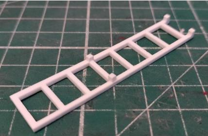
**Step 23:** The ladder can be constructed by gluing the four small blocks 42 to the back of the ladder 36. The ladder can be glued to the front before or after painting. Better paint coverage is achievable when left off. Glue one set of blocks to the turreted end and then 4 rungs further down.
