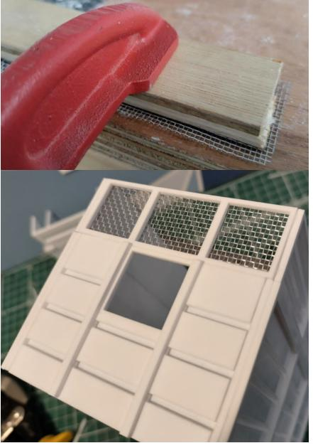
If building the silage variant also glue the mesh to 37. You may need to apply some pressure to the mesh while gluing to obtain a strong bond. You can see how we have used a clamp and some wood to hold the two together while the glue sets. Do NOT overtighten or the acrylic plastic will break.
