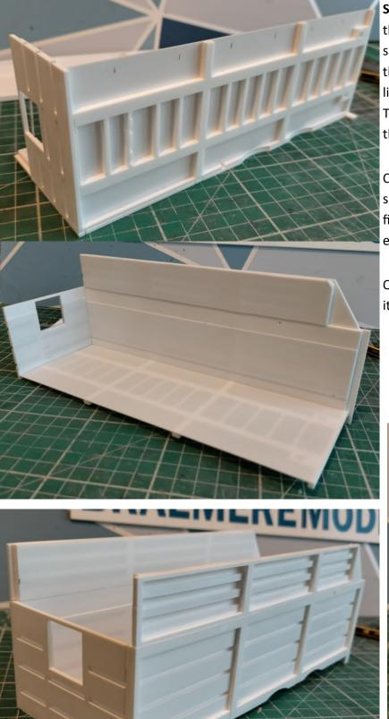
**Step 17:** To build the body first glue one side, the front and the floor together to create a square corner. The front fits in the recess at the front of the side. The bearers in the floor line up flush with the bottom of the sides. The thin floor sheet should sit just above to the two curved wheel cut outs.
