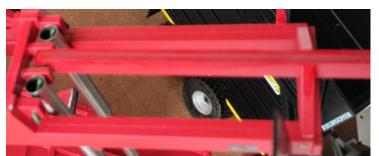
**Step 9:** Fit the drawbar. Loose fit the axles and wheels to the chassis. Select the tractor you wish to hook the trailer too. Place the drawbar eye on the tractor hitch, position the drawbar in the trailer as shown and glue a pin in the appropriate hole on the drawbar hanger. This will allow the trailer to sit correctly on the tractor.
