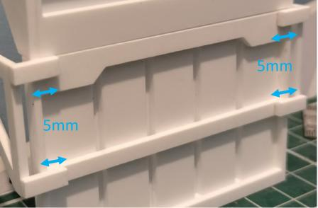
**Step 20:** Constructing the rest of the tailgate by gluing tabs 38 to either side of the tailgate, one at the top an one in the middle as illustrated, they glue 5mm in from the side with the remainder overlapping. They tabs sit up to the raised edge of the border and the narrower spacing sits to the top of the tailgate.
