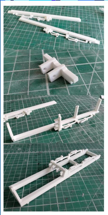
**Step 2:** Glue the two halves of the chassis rails together. 17 to 18 aligning the pivot hole at the rear and the dropped mount in the middle. Take care if using superglue, the bond will be almost instant so make sure they are aligned as you glue. Ensure you glue them opposite sides to make the offside and nearside chassis rail
