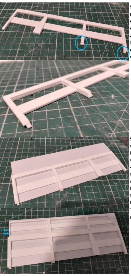
**Step 10:** To begin constructing the body glue the side panels together. 1 onto 2, ensure you glue one side opposite to the other!
