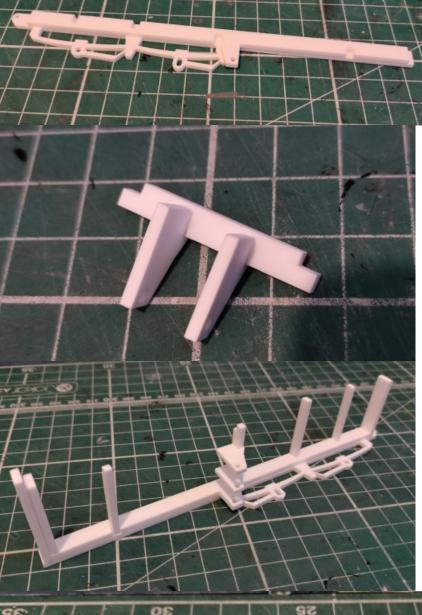
**Step 2:** Glue the two halves of the chassis rails together. 16 to 19 aligning the lengths and set the inside (19) 3mm back from the front. Take care if using superglue, the bond will be almost instant so make sure they are aligned as you glue. Ensure you glue them opposite sides to make the offside and nearside chassis rail
