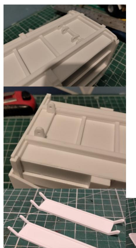
**Step 20:** Add the under body pins. The ram pins 33 glue into the slots in cross member. Ensure the holes point to the back of the body.
